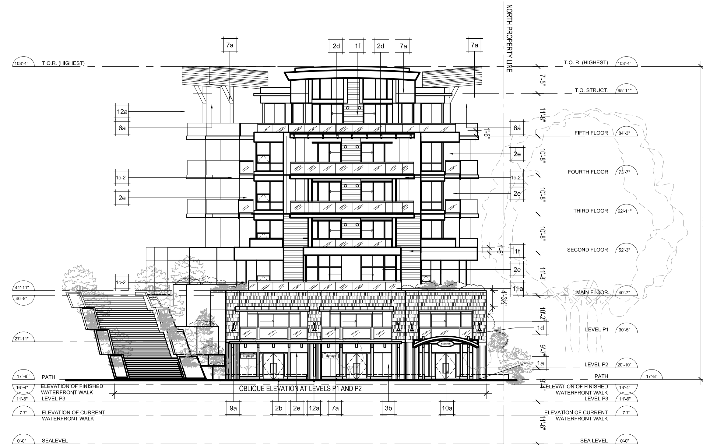
RESIDENCES - EAST ELEVATION FROM SEAWALK SCALE: 1/16"=1'-0"
