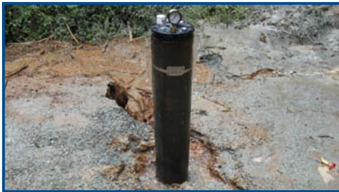
Figure 3. Erosion caused by flowing artesian well.
