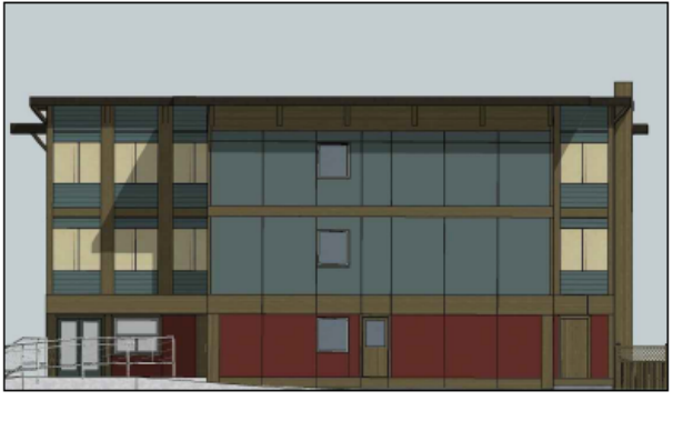
3. fibre cement board panel siding
