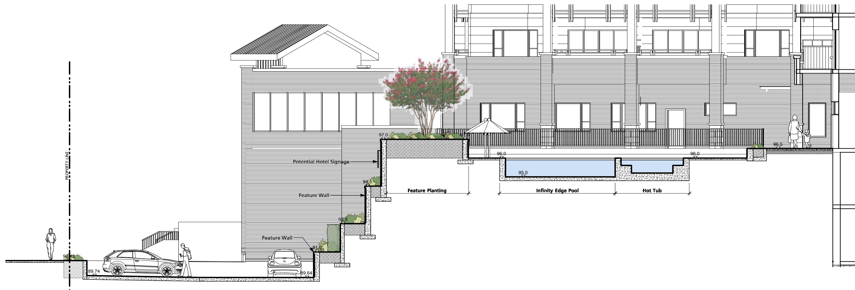
6 SECTION A THROUGH RETAINING WALL AND INFINITY EDGE POOL 1:100
