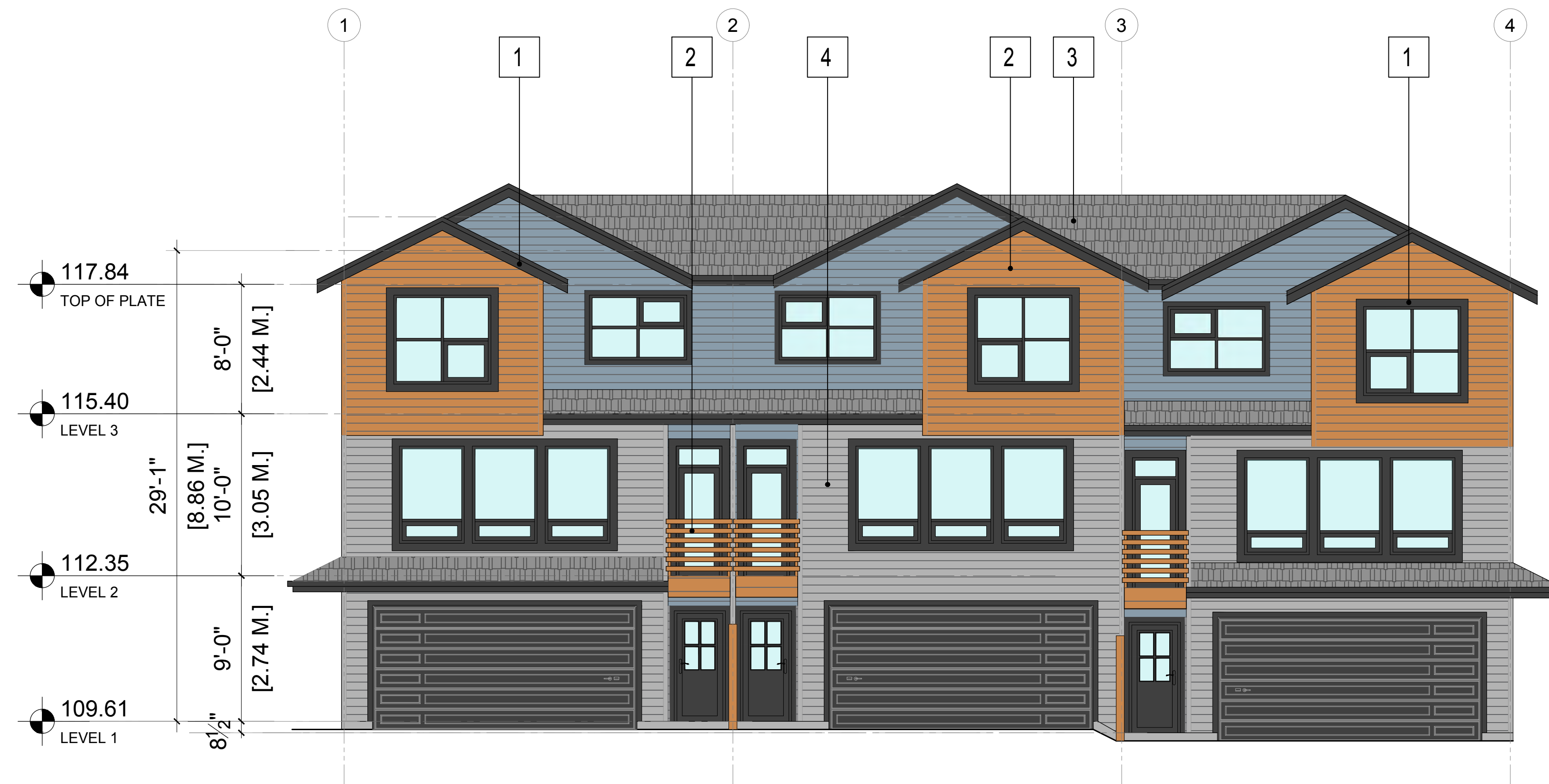
1 BUILDING 6 - SOUTH ELEVATION SCALE : 3/16" = 1'-0"
