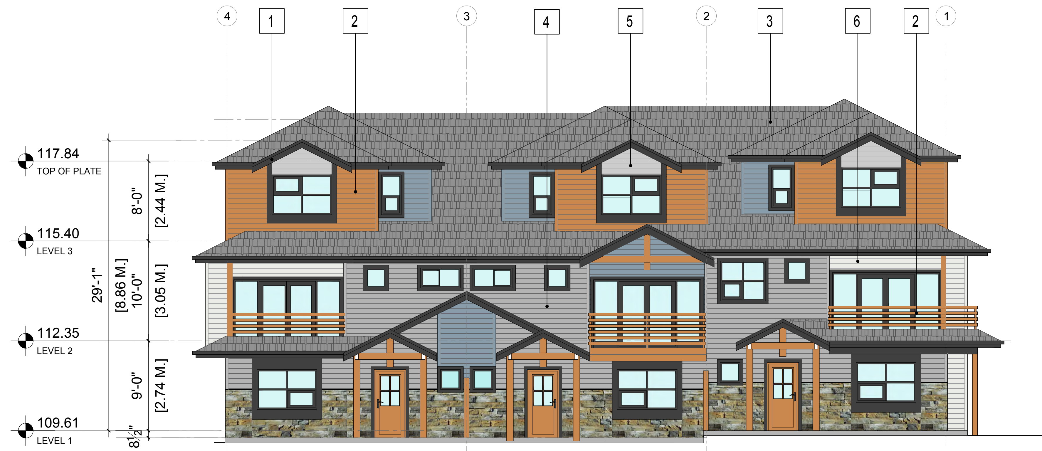
1 BUILDING 2 - NORTH ELEVATION SCALE: 3/16" = 1'-0"
