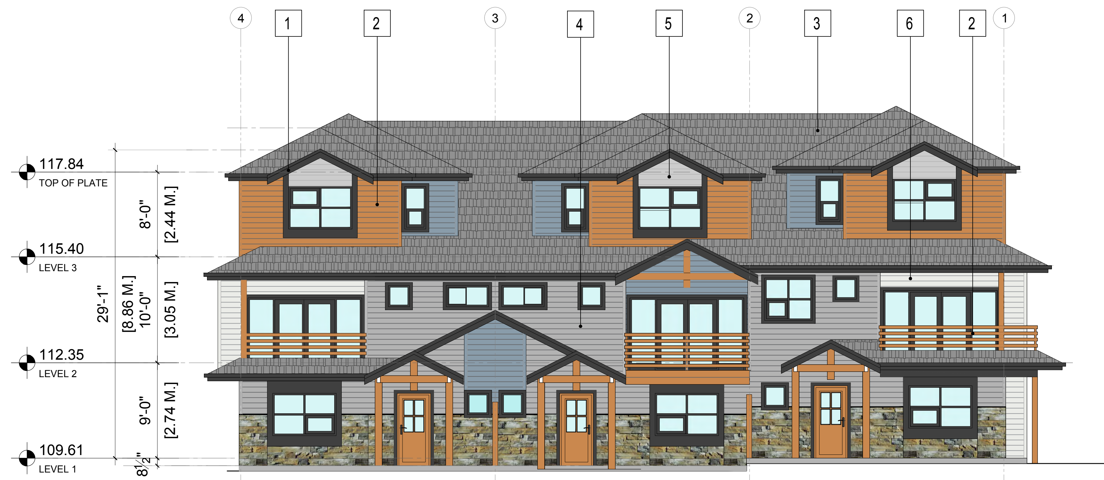
1 BUILDING 1 - NORTH ELEVATION SCALE : 3/16" = 1'-0"
