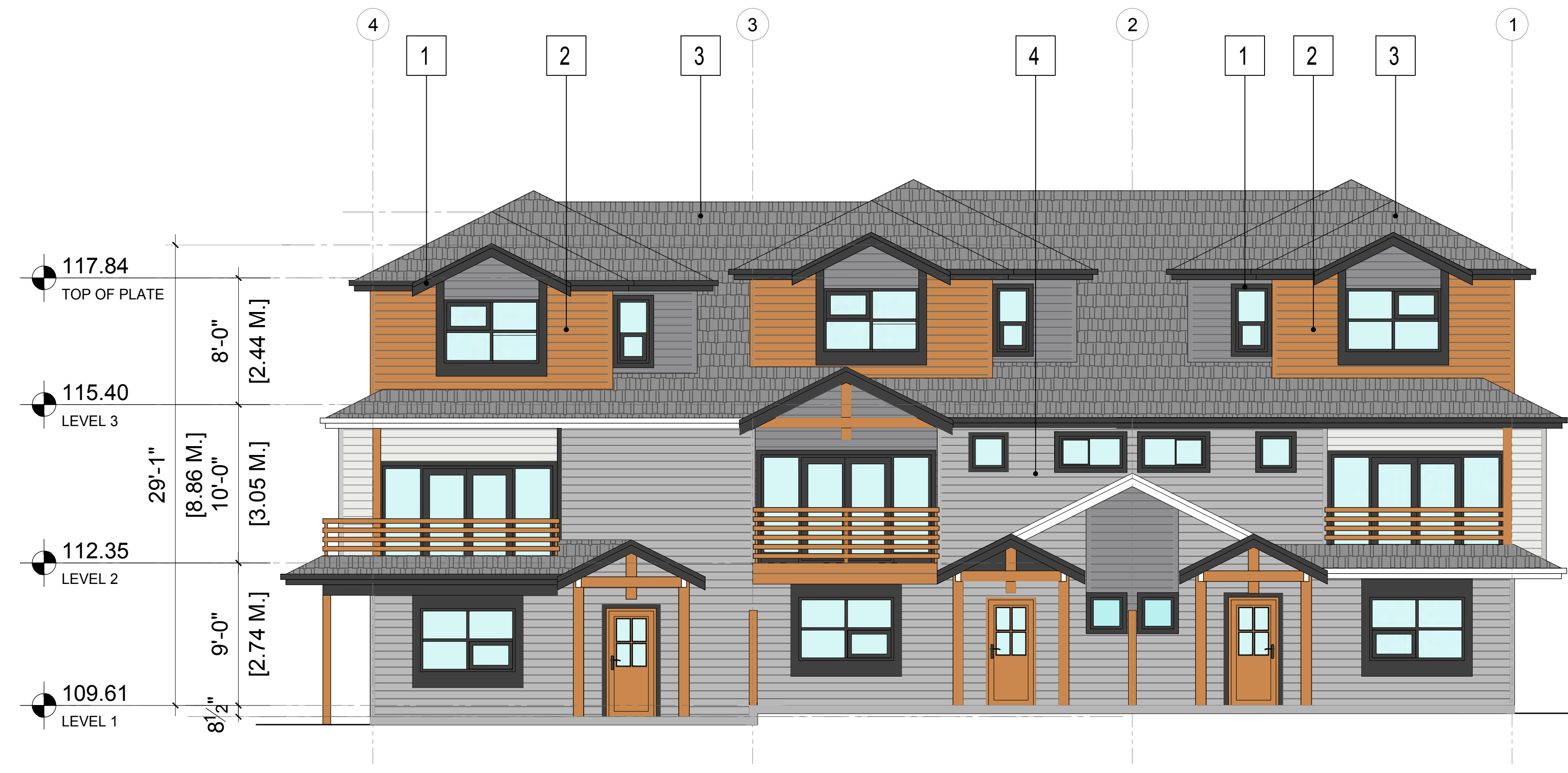
1 BUILDING 6 - NORTH ELEVATION SCALE : 3/16" = 1'-0"
