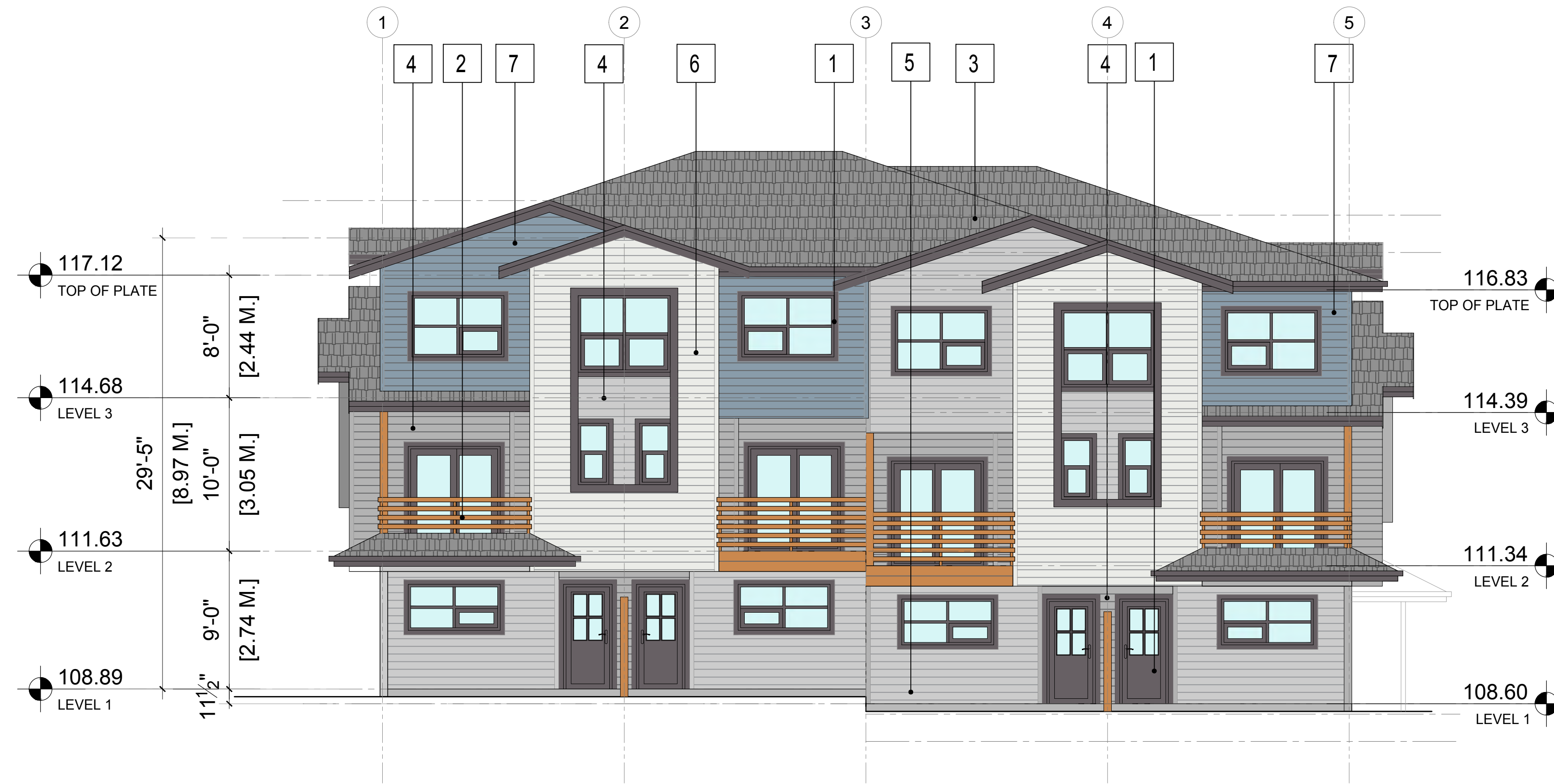
3 BUILDING 3 - NORTH ELEVATION SCALE : 3/16" = 1'-0"
