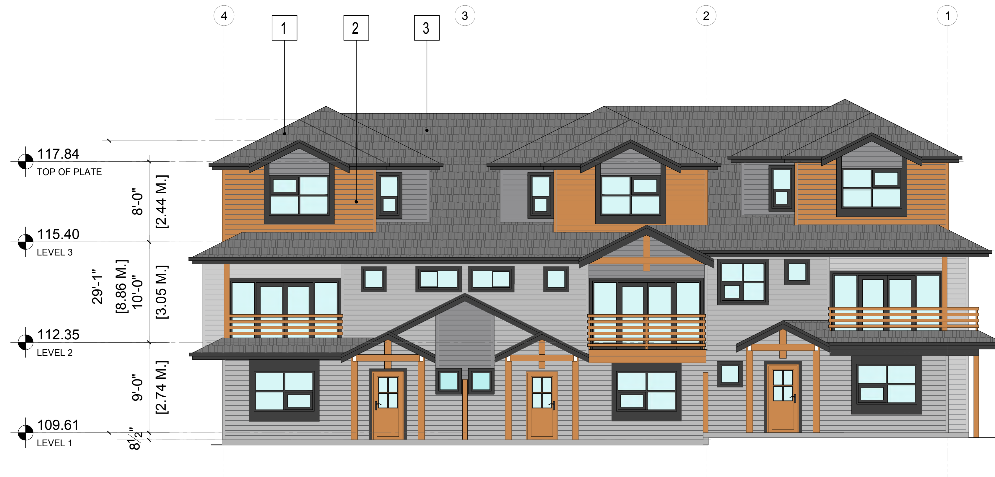
1 BUILDING 5 - NORTH ELEVATION SCALE : 3/16" = 1'-0"
