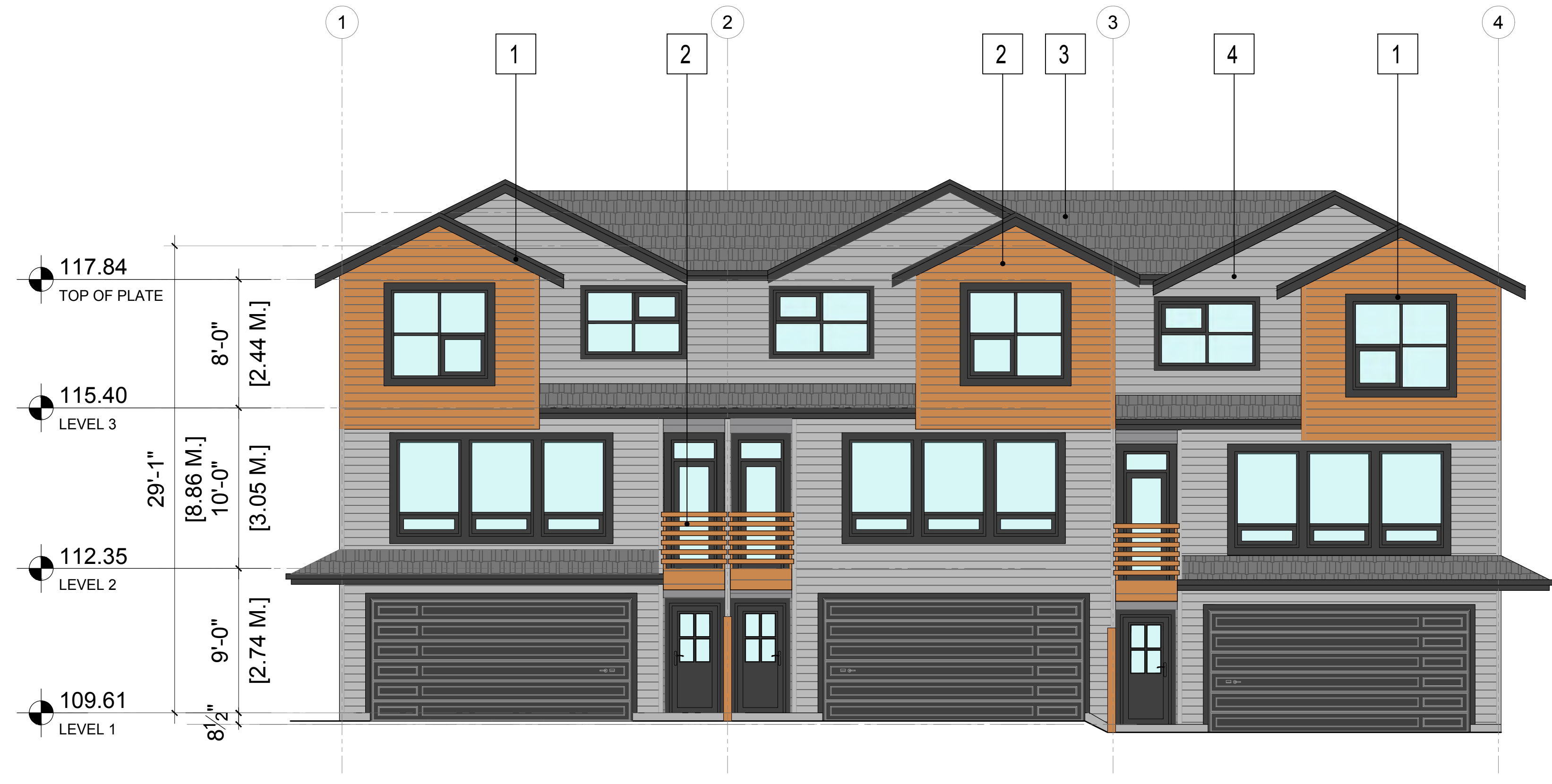
1 BUILDING 2 - SOUTH ELEVATION SCALE : 3/16" = 1'-0"
