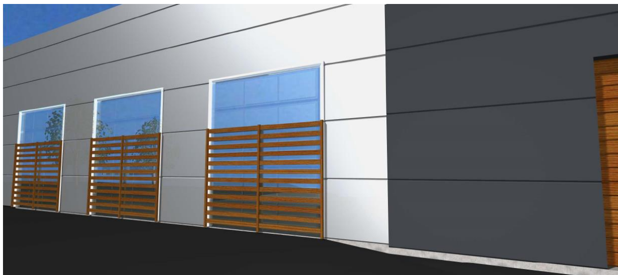
WOOD SCREENS PROVIDE SECURE VENTILATION FOR EMPLOYEE WORK AREAS
