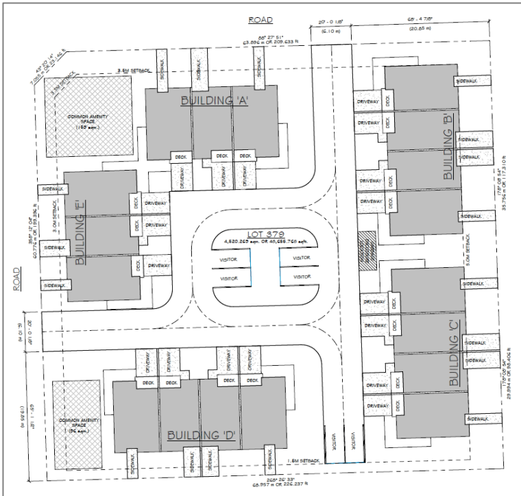
Figure 2: Proposed site plan for Lot 37 showing three four-unit townhouse buildings and two three-unit townhouse buildings for a total of 18 dwelling units
