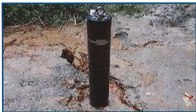
Figure 3. Erosion caused by flowing artesian well.
