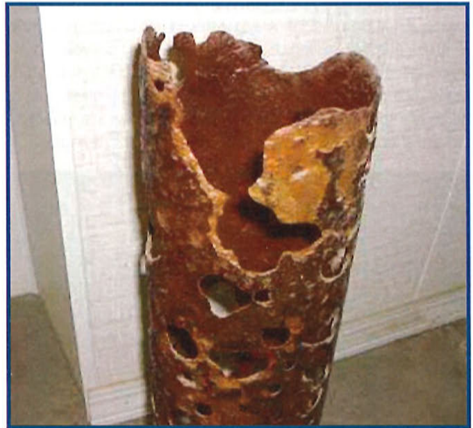
Figure 5. Corroded well casing.
