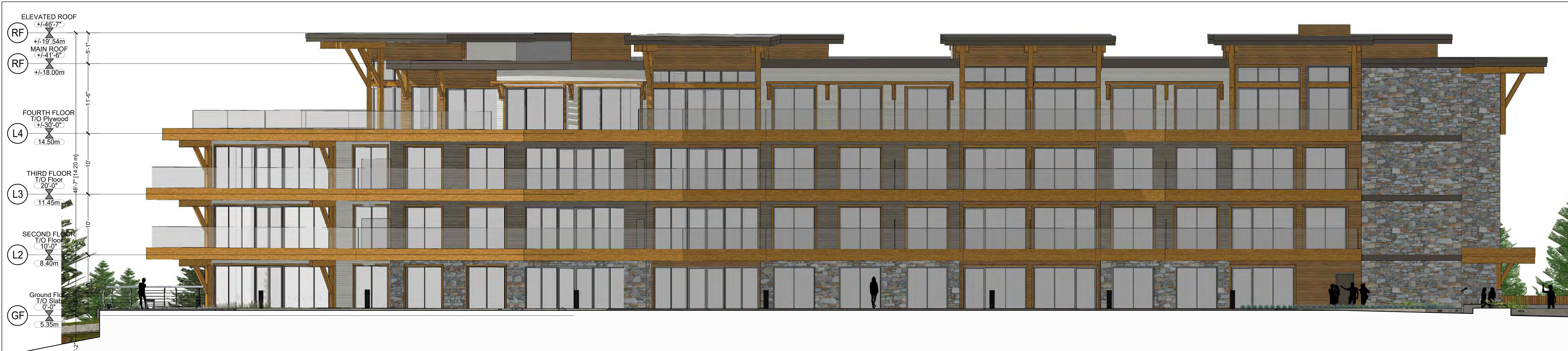
2 BUILDING B - NORTH ELEVATION Scale: 1/8" = 1'-0"
