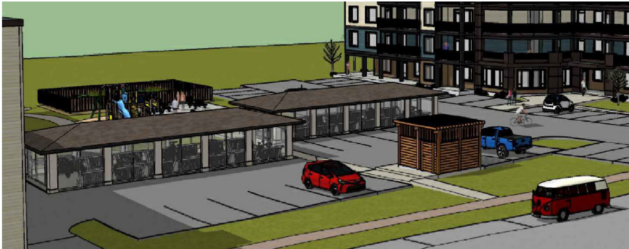
Figure 4 - Bicycled 'shed' parking structures required to meet bylaw requirement and store 95 bicycles. The applicants request to reduce the bike parking requirement to reduce the size of the structures within the courtyard.
