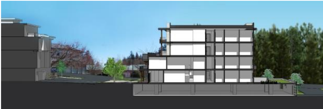
Figure 2: Cross-section (west) of the building, showing the four storeys and elevation change of the lot.
