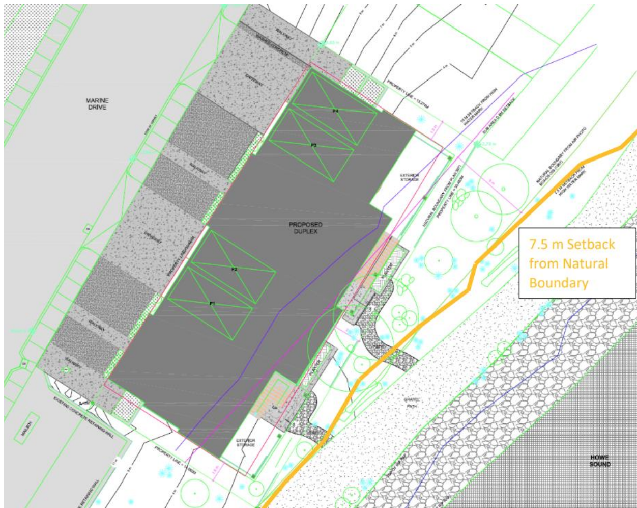
Figure 8: Plan view of the proposed development- 7.5m setback from Natural Boundary highlighted in Yellow.
